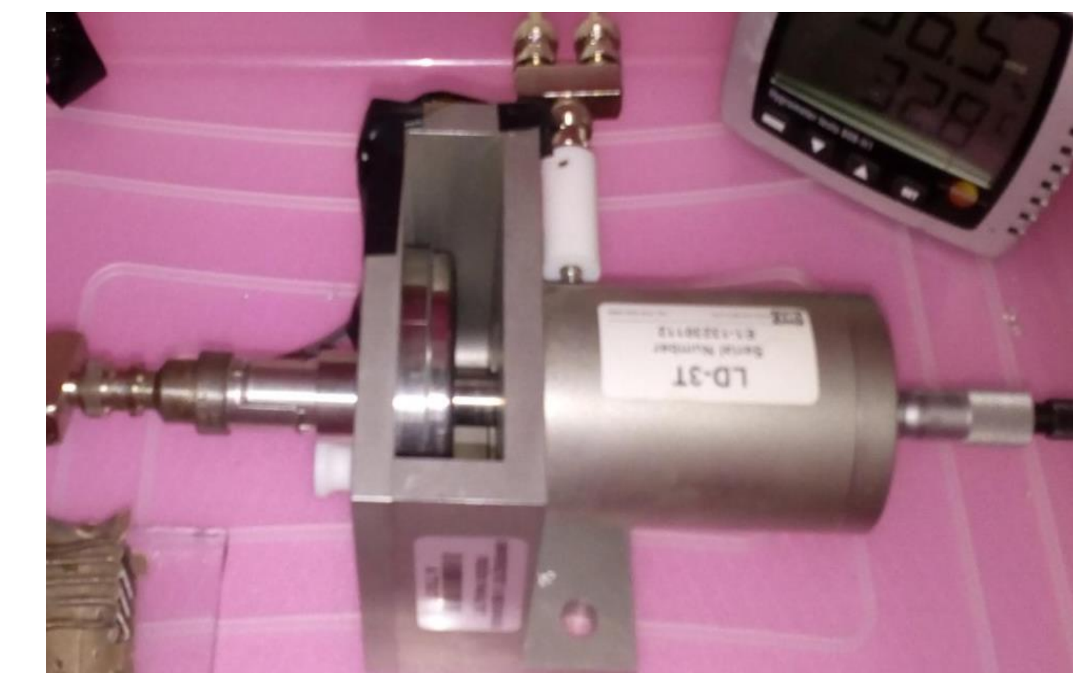
Figure 2. LD-3 Rigid Dielectric Cell for dielectrical measurements.
