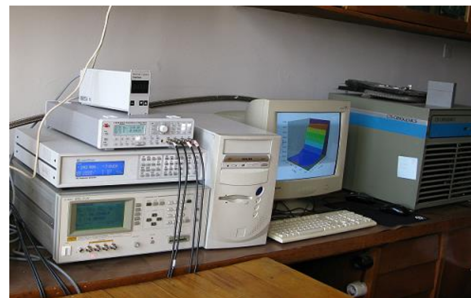
Figure 1. Experimental setup for a measuring of the dielectric properties.
