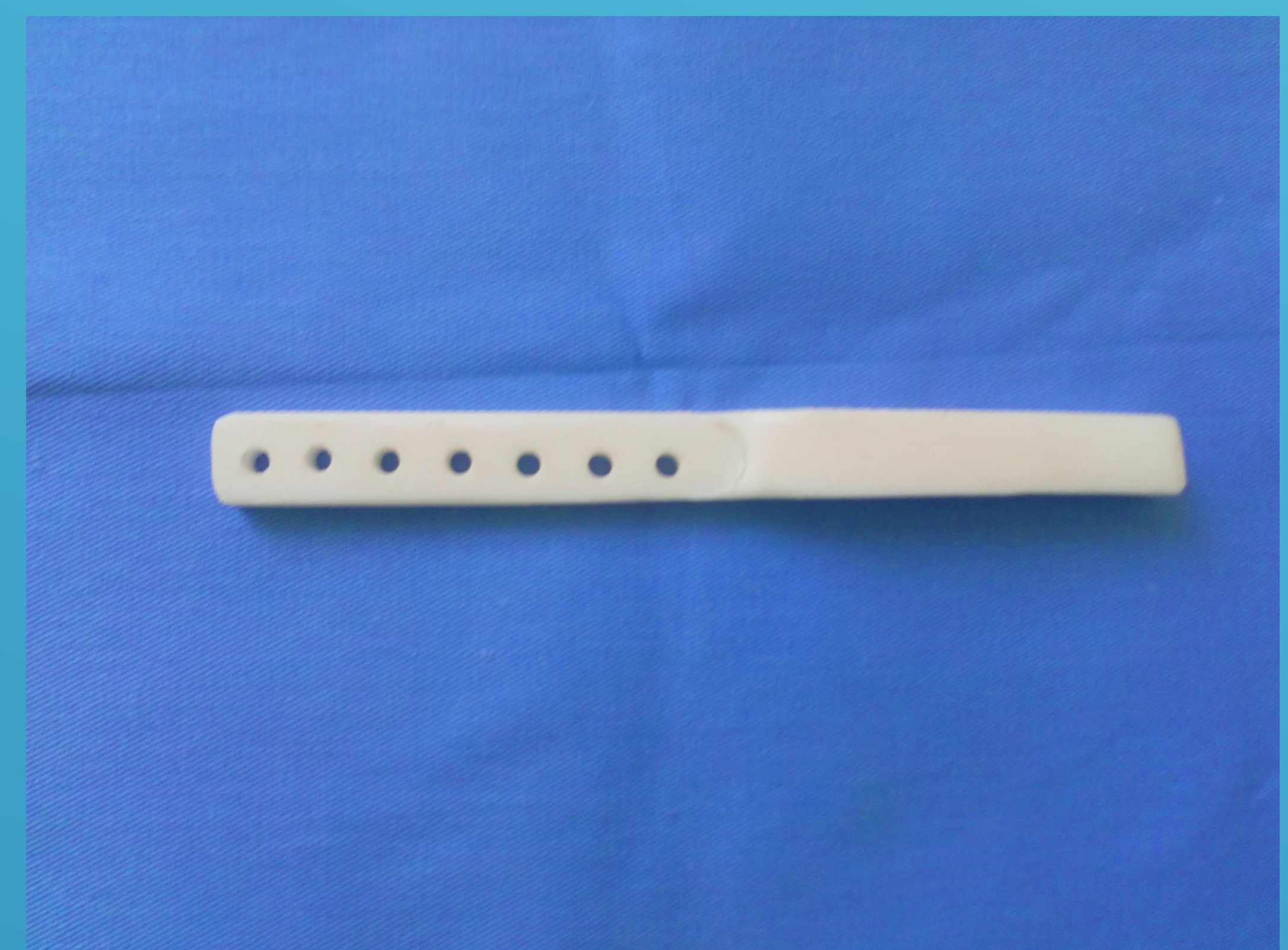
Fig. 1. Specially designed Teflon mold for making samples
