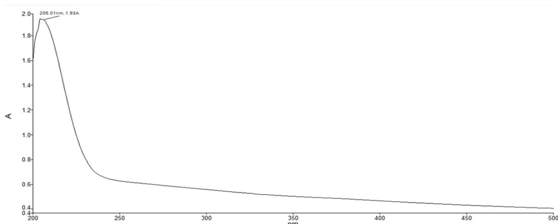
Figure 2. UV-Vis spectra of Zinc oxide nanoparticle in the range 200 - 500 nm
