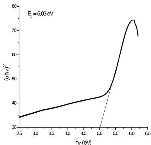
Figure 3. The Tauc plot of ZnO nanoparticles
