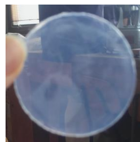
Figure 5. Nano-cellulose dispersion and nano-cellulose film obtained from TEMPO-oxidized cellulose
