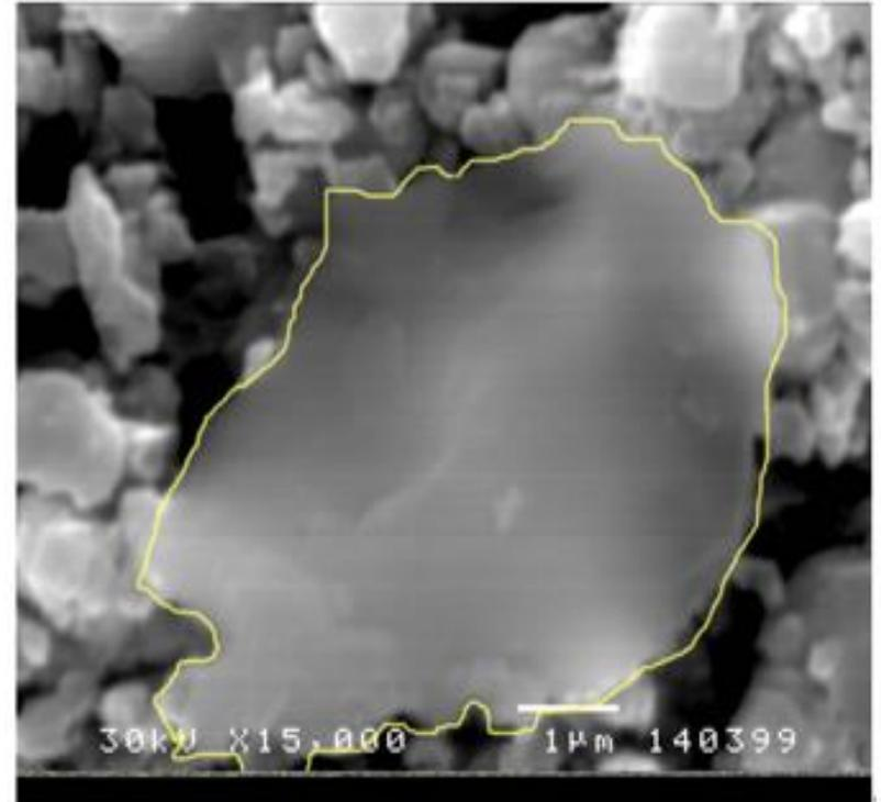
Figure. Microstructures of  $\text{BaTiO}_3$ -ceramics and fractals reconstructing the perimeter of the grain.
