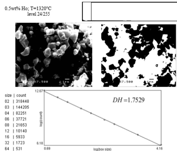
Figure. BaTiO<sub>3</sub>-ceramics sample and its fractal dimension.
