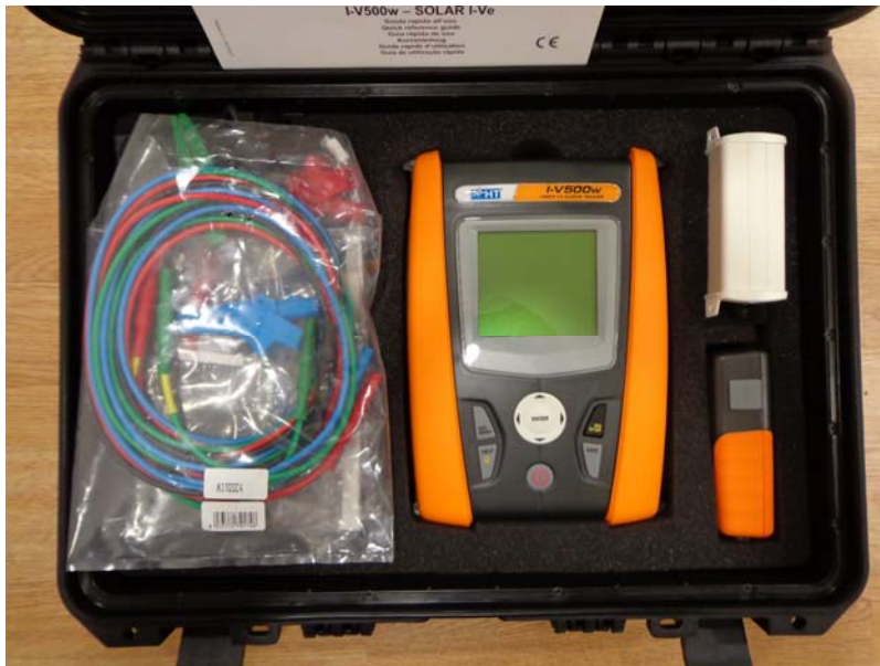
I-V curve meter DC voltage up to 1500 V
