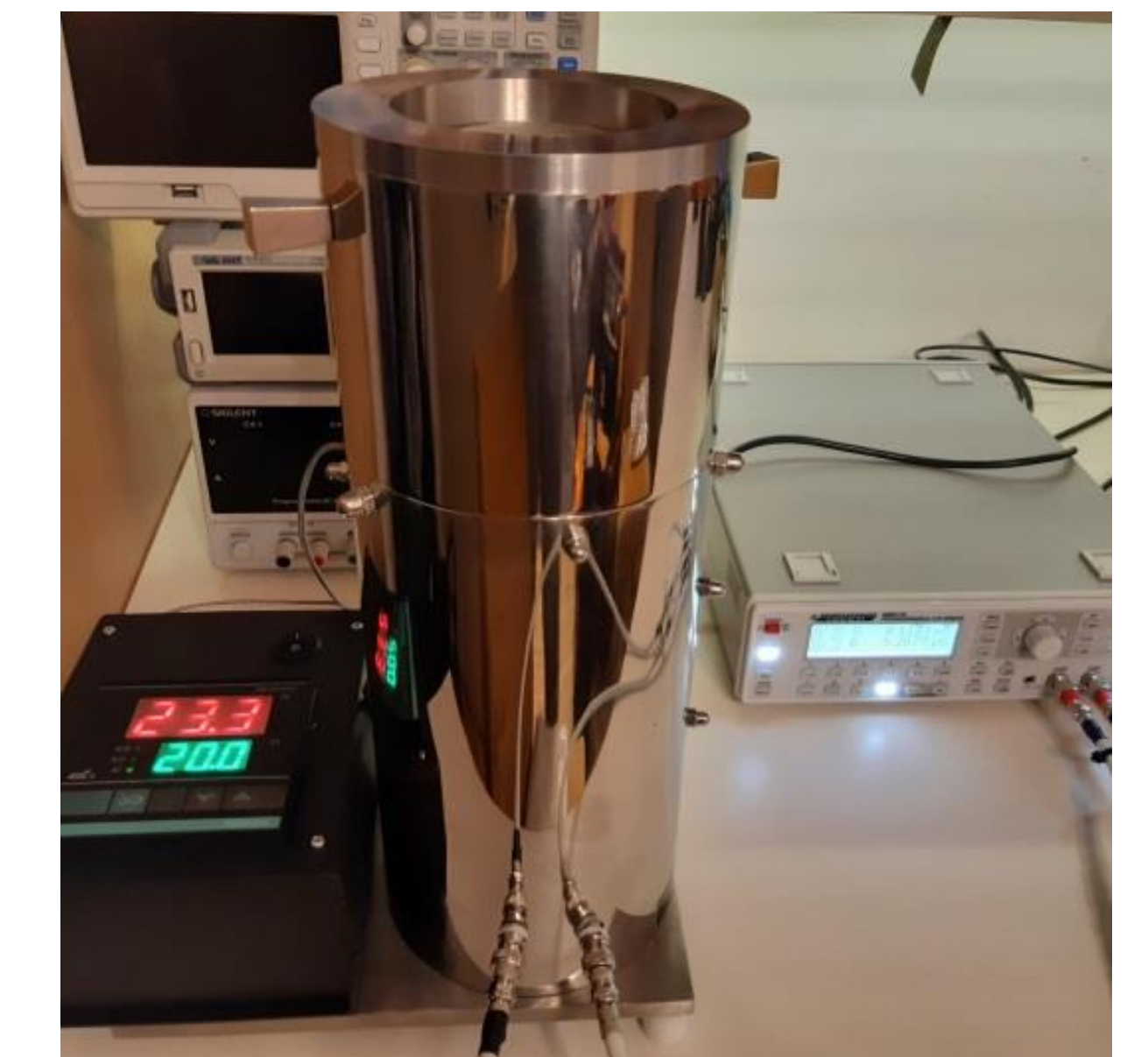
Figure 2. Experimental setup for a measuring of the dielectric properties of fabrics.
