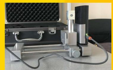
Determination the range of Alpha particles with (Am-241) energy about 4 MeV in air using pixel detector.
